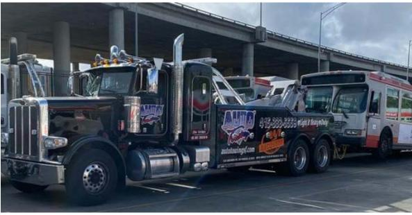
The Auto Towing wrecker shown is towing an articulated bus. These wreckers are capable of towing large vehicles such as big rigs, fire trucks, buses, etc. The cost of a wrecker like the one shown can be \$500k to \$750K.
